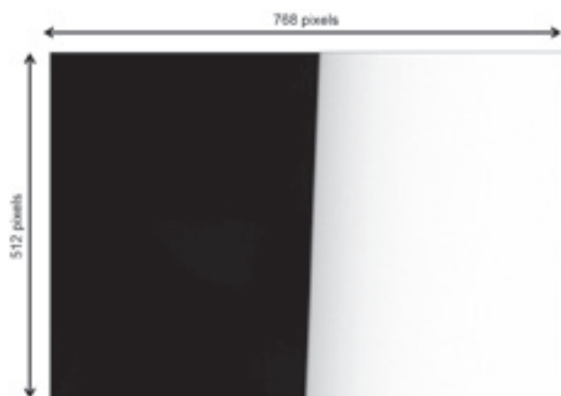
Fig. 2 Example ROI image obtained from the experimental edge image. The right side shows the tungsten edge device with a slight angle.
