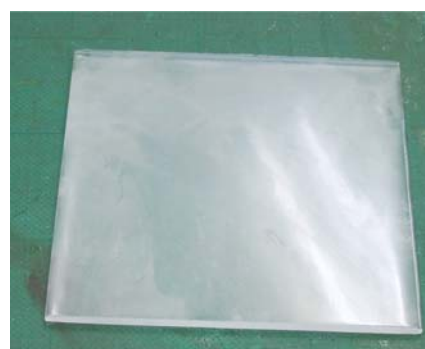
Fig.2 EVA plate around in 6mm thick and 100mm square can be purchased as the dental material for the mouth piece as the sport mouth guard.
