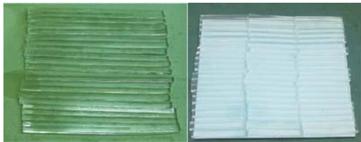
Fig.4 The squid roa fish like strip food model(Left) for the sagittal biting fringe observation slitted from EVA plates of 100mm square and strips were cut into three short billet for laminating food models (Right).
